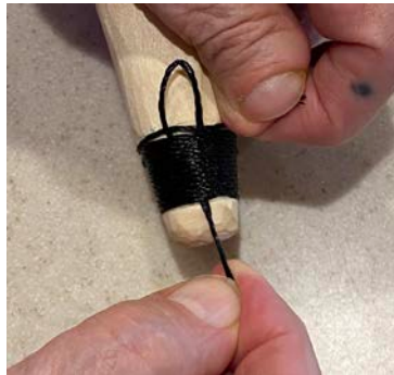
Keeping the wrapping tight, I pulled the free end of the loop.
