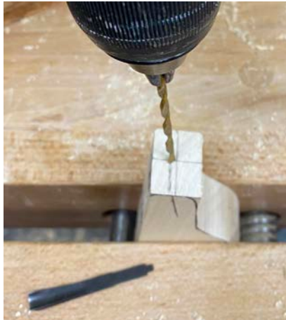
Drilling on an Angle
