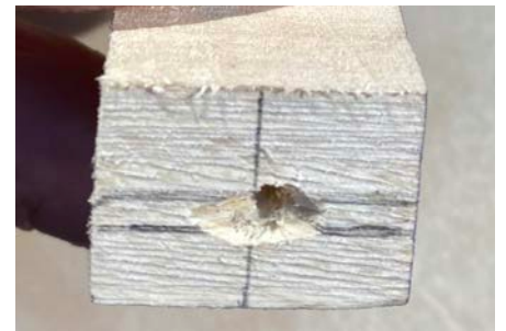
Hole With Notches Was Off-Center
