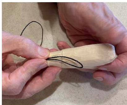
Using 1mm tarred nylon twine, I placed a loop overlapping the tapered notch
