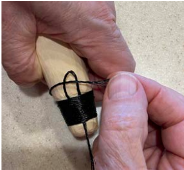
When the notch area was covered, I threaded the twine through the loop.
