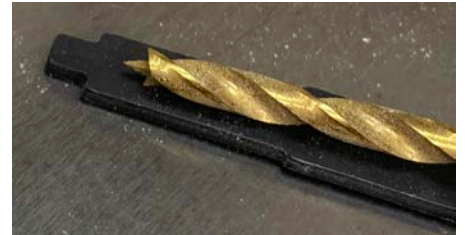
Drill Slightly Smaller than Blade
